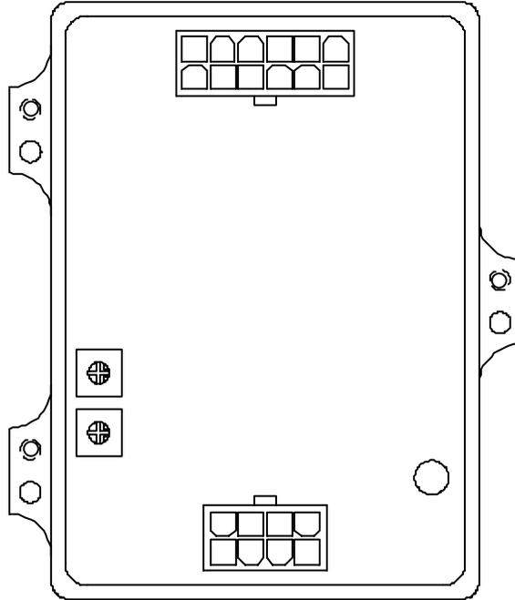
20. There is a 12-pin connector housing at the “top” of the module, 8-pin housing at the “bottom” of the module, two blue potentiometers, and a red LED. Use a piece of string or wire or tape or a tie-wrap to temporarily suspend the module somewhere near the alternator assembly, so that you can see both the alternator stator’s timing marks and the module’s red LED in your field of vision at the same time.
