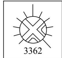
If you look carefully at the potentiometer, you'll see the markings "3362" along one edge, and engraved position markers around the adjustment screw. The screw has a small relieved area that shows where it is set.
