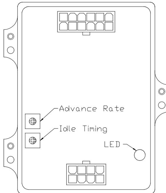
33. When you mount the module, it is handy to have screwdriver access to these potentiometers. The idle-timing potentiometer is pre-set at the factory, but may be varied by those who prefer more or less idle-speed advance than standard. The advance-curve rate is pre-set at the factory to be all-in (full advance) at 3,250 RPM, but is adjustable to be all-in anywhere between 3,000 and 4,000 RPM. Directions on how to adjust both of these controls are included in Appendix 1 of these instructions.
