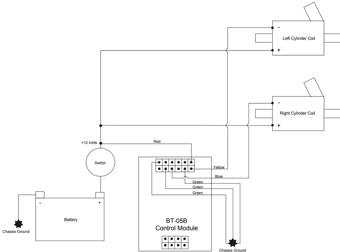
43. Once you've got the pickup plate wire harness and the power cable harness wiring and routing complete, plug the two connectors into the control module.
