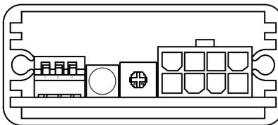
20. There is an 8-pin connector toward the right side of the module, a three-position DIP switch toward the left side, and a red LED and blue potentiometer between the two. There is also a 6-pin connector (not shown in the line drawing) at the end of a short wire bundle coming out the module. For the next steps, statically timing the system, temporarily suspend the module somewhere near the alternator assembly, so that you
