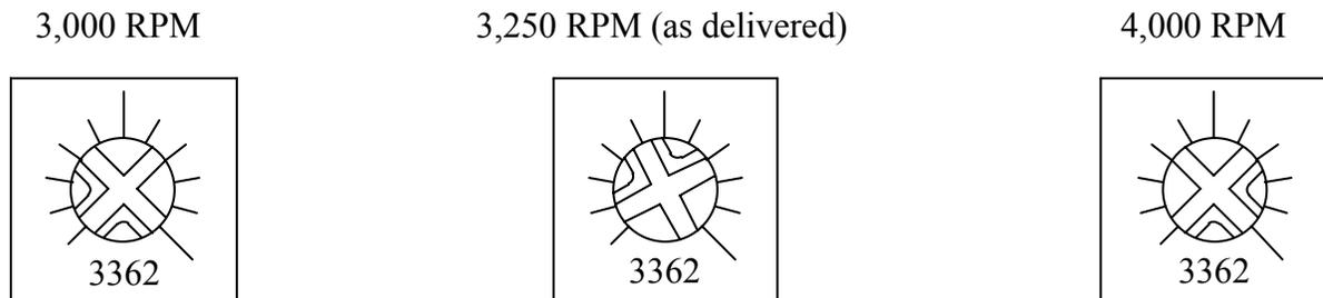
If you look carefully at the potentiometer, you'll see the markings "3362" along one edge, and engraved position markers around the adjustment screw. The screw has a small relieved area that shows where it is set.
