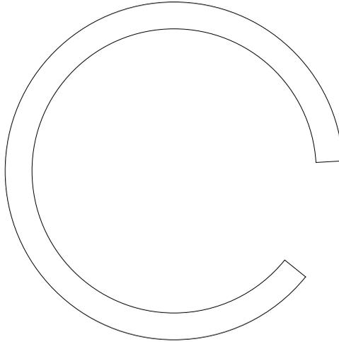
18. Slip the spacer gap around the wire bundle behind the pickup plate, and install the spacer in the original points-plate relief in the housing, oriented as shown in the drawing above (the gap in the spacer straddles the exhaust rocker-shaft locknut).
