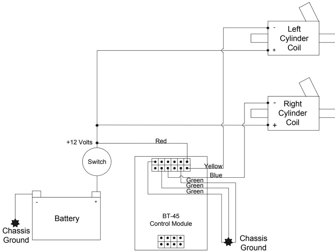
56. Once you've got the pickup plate wire harness and the power cable harness wiring and routing complete, plug the two connectors into the control module.
