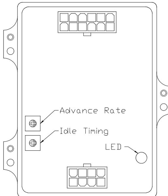
33. There is a 12-pin connector housing at the “top” of the module, 8-pin housing at the “bottom” of the module, two blue potentiometers (one for adjusting the
