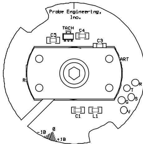
29. Check to make sure the alternator rotor mark is still aligned with the "T" mark on the stator housing. If the crankshaft position moved while you were tightening the rotor's expander screw, loosen the rotor and repeat steps #26 and #28 until everything looks right.
