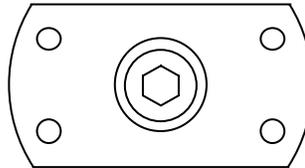
23. Using a 3/16” hex wrench, loosen the internal-expander screw inside the trigger rotor a couple of turns, then slip the rotor into the freshly cleaned left-side bore of the camshaft until the rotor bottoms on its shoulder. Spin the rotor inside the camshaft a few turns to ensure that it doesn’t foul the pickup plate’s wires (or anything else). Don’t tighten the internal-expander screw yet.
