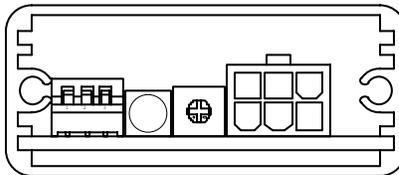
34. There is a 6-pin connector toward the right side of the module, a three-position DIP switch toward the left side, and a red LED and blue potentiometer between the two. There is also a 5-pin connector (not shown in the line drawing) at the end of a short wire bundle coming out the module.
