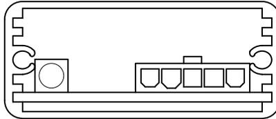
14. There is a 5-pin connector at the right side of the module (into which the pickup plate lead-wires plug) and a red LED at the left side. There is also a 4-pin connector (not shown in the line drawing) at the end of a short wire bundle coming out the module; this connects to the Power Cable Harness.
