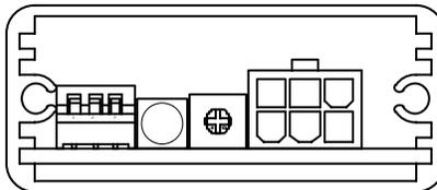
24. There is a 6-pin connector toward the right side of the module, a three-position DIP switch toward the left side, and a red LED and blue potentiometer between the two. There is also a 5-pin connector (not shown in the line drawing) at the end of a short wire bundle coming out the module.
