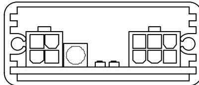
24. There is a 4-pin connector at the left side of the module and a 6-pin connector at the right side; between the connectors are a red LED and a pair of micro pushbuttons.
